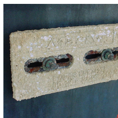
Unprotected and premature transom & outdrive zinc loss
