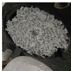
Unprotected and premature transom & outdrive zinc loss
